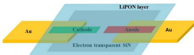
**Figure 1.** Schematic shows the general concept of the proposed *operando* TEM nanobattery setup. The MEMS-based TEM chip acts as a platform where the nanobattery comprising of a single-particle cathode, anode and thin solid-state electrolyte can be assembled.
