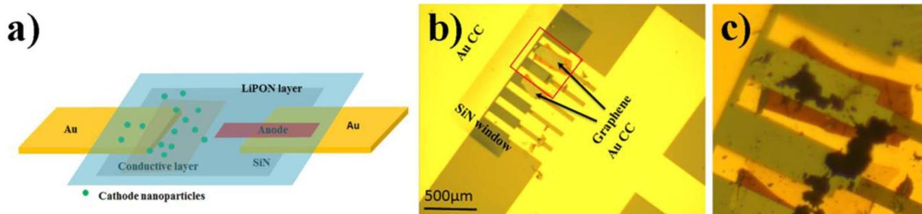
**Figure 3.** (a) Schematic showing the principle of the nanoparticle battery system; (b) Graphene flakes are transferred on the electron transparent SiN window of the MEMS chip; (c) zoomed in image of the rectangular area marked with red line in (b) after LiFePO<sub>4</sub> dispersion and LiPON deposition.
