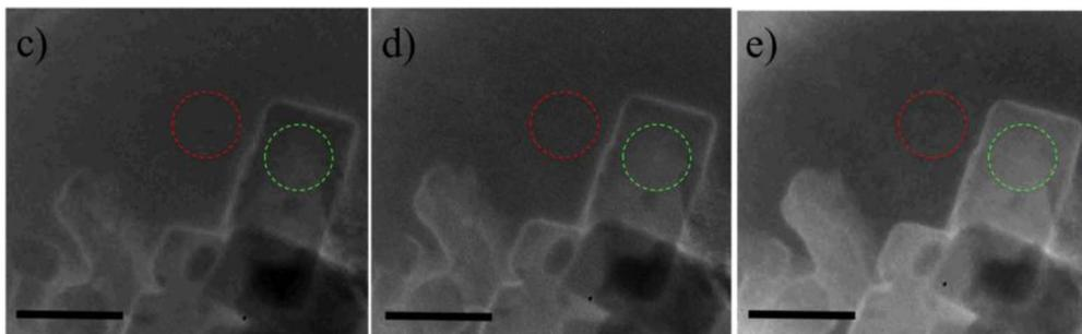
**Figure 4.** EFTEM images of the LiFePO<sub>4</sub> nanoflakes during different stages of charging, acquired with a 5 eV slit at 5 eV: (a) before applying bias, (b) after 150s of charging, and (c) after 300s of charging. The scale bar is 200 nm. The area indicated by green and red dotted circles are used to measure the intensity variations on and off the LiFePO<sub>4</sub> particles respectively and are listed in Table S-2.
